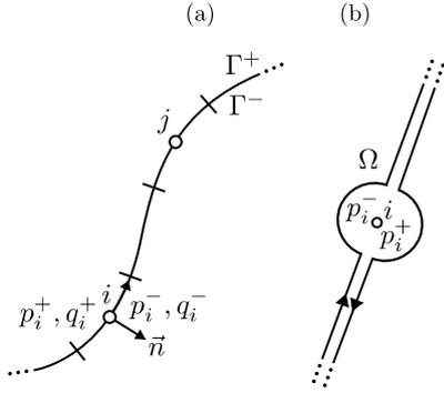
Image 1. (a) Geometric idealization as single-wire configuration of a barrier featuring a very thin section. (b) Strategy used to avoid the singularity around the collocation point in the dual approach for the treatment of elements idealized as null-thickness type
