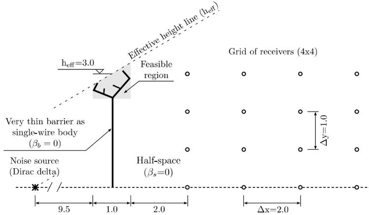
Image 2. Bi-dimensional configuration for the MO optimization of the topological barrier design under study. Dimensions expressed in meters
