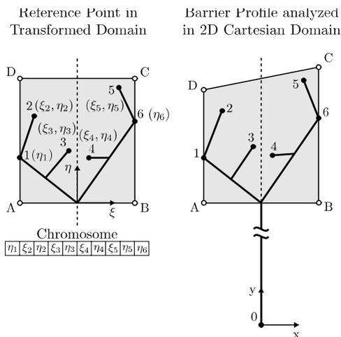
Image 4. Model under study. Y-variant-shaped barrier with six design points
