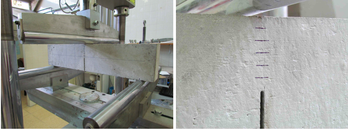
Figure 1: Specimen during a three-point flexural test (left) and detail of cracks after test (right).
